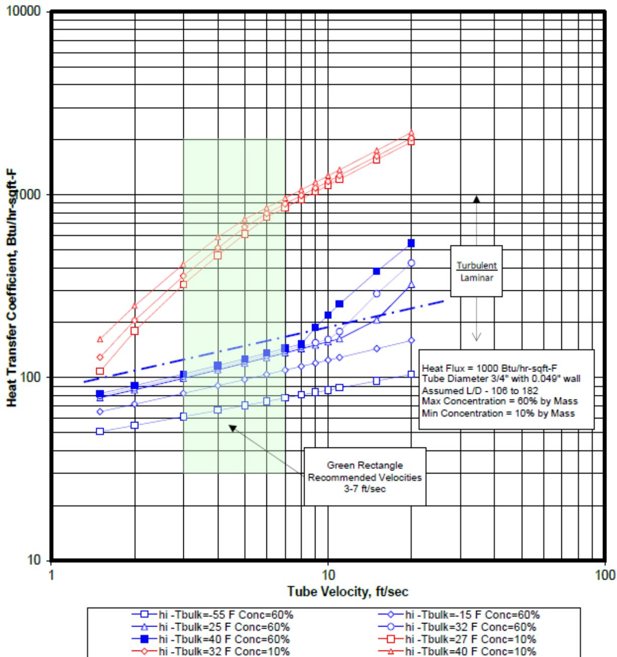
Figure 3. In-Tube Heat Transfer for Propylene Glycol-Water Solutions
