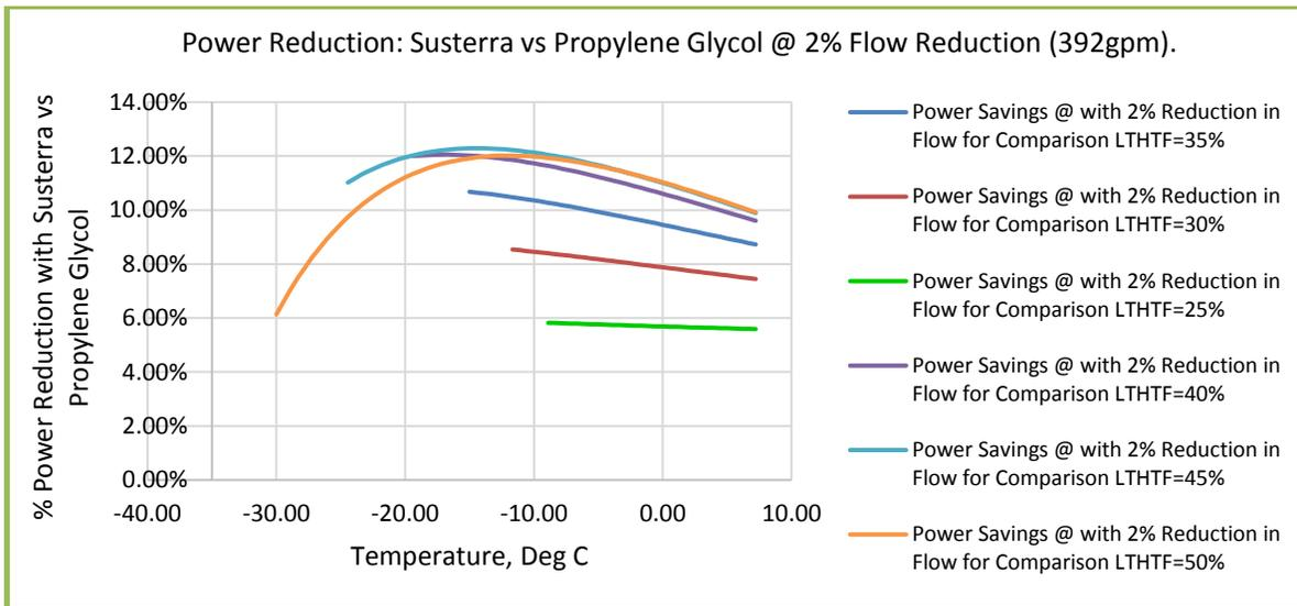
**Figure 8. Pump Power Reduction: Susterra® Propanediol-Water vs Propylene Glycol-Water Solutions at 2% Flow Reduction.**
