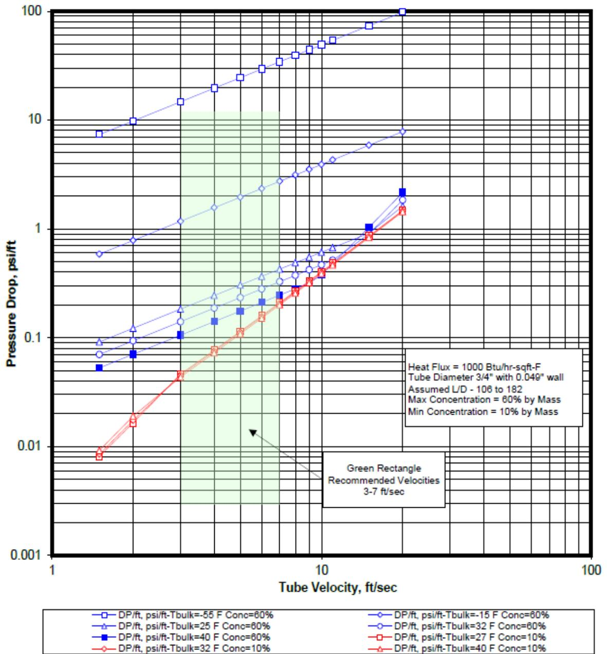
Figure 5. In-Tube Pressure Drop Propylene Glycol-Water Solutions
