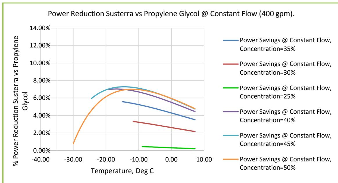
**Figure 7. Pump Power Reduction: Susterra® Propanediol-Water vs Propylene Glycol-Water at Constant Flow**
