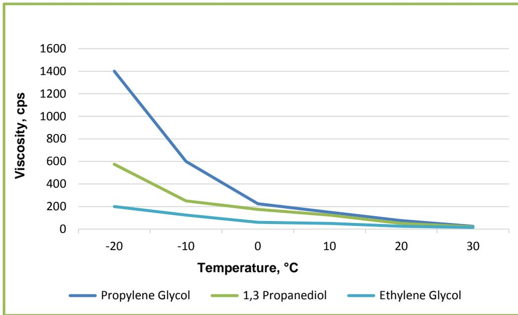
**Figure 1: Viscosity profile of glycols as function of Temperature**
