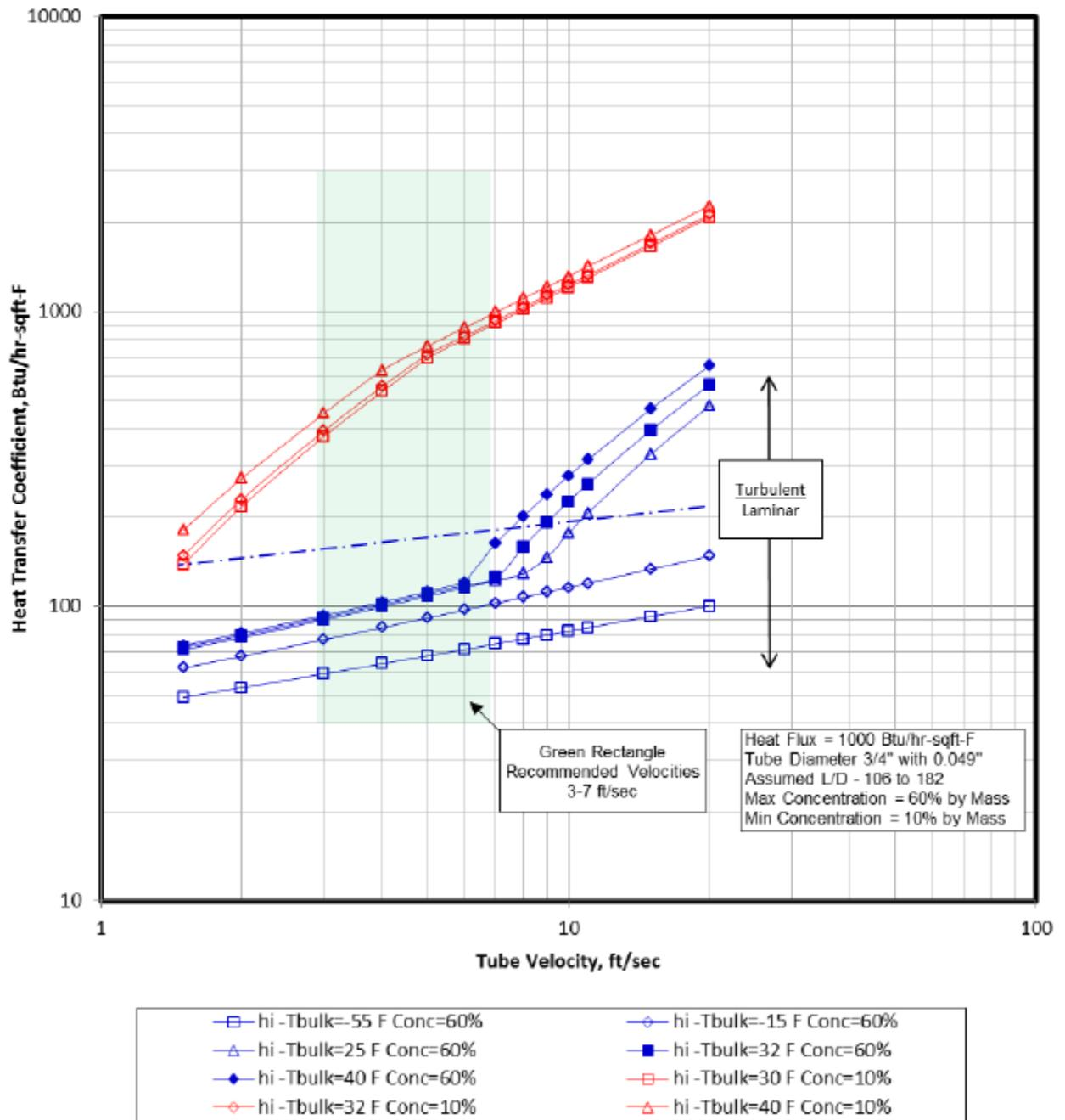
Figure 2. In-Tube Heat Transfer for Susterra® Propanediol-Water Solutions
